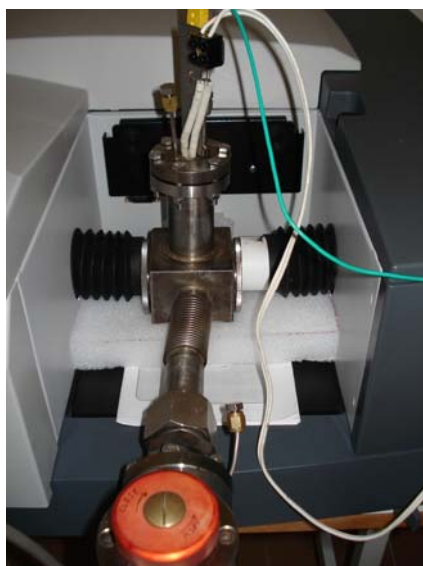
Variable temperature (-190- 450 °C) cell for in situ study of catalysts.
