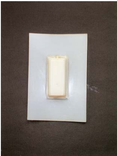
Commercial full polyethylene-body cell with different (0.5-2.5 mm) thickness
