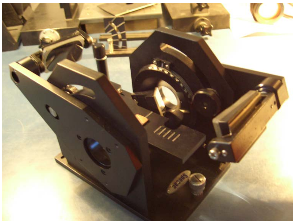
Special optical accessory for RAIRS measurements
