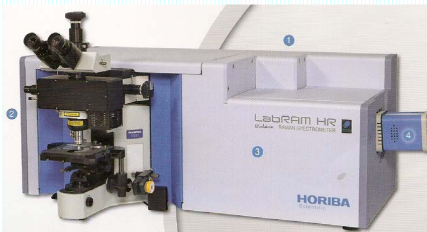
General view of Horiba Scientific LabRAM HR Evolution Raman microscope spectrometer (SU), \lambda_0= 532, 633, 785\text{nm}
